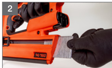
2 Make sure top of head aligns with Head supporting Brad Channel
