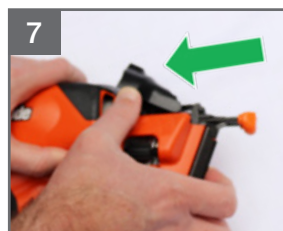
7 Clip nose plate cover assembly pin over nose location studs #64
