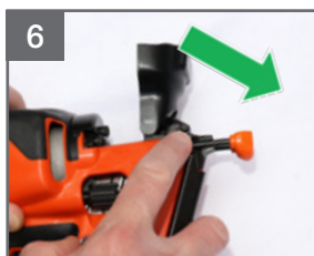
6 Close nose plate assembly #60
