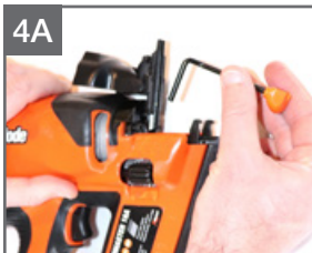
4A Only if needed to clear jam - remove No Mar Contact Probe #62 & 63
