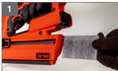
1 Insert selected brads into magazine
