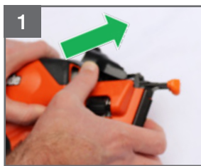
1 Lift nose plate cover to release nose plate assembly #60
