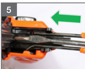
5 Verify driver piston assembly #22 is returned to top position prior to firing tool
